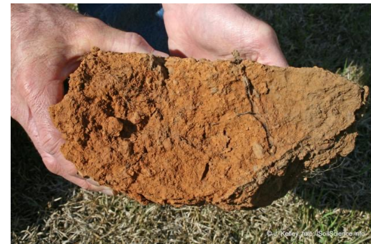
Prismatic Structure - prisms are 35 to 45 mm across.
