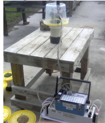
Figure 9. Portable chamber system for measuring canopy gas exchange.
