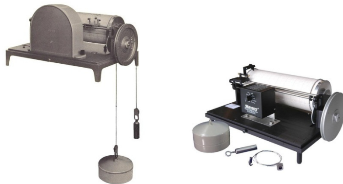
Figure 2. Left: A Stevens Type F Chart Recorder from the 1960's, which was used in many USGS Stream Gaging sites. Right: The current production model of the Stevens Type F Chart Recorder [Stevens 12].
