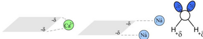
Figure 4. Planner clay lattice: a negative charge distribution [left]; cation influence [center]; and Dipole moment of a water molecule [extreme right].
