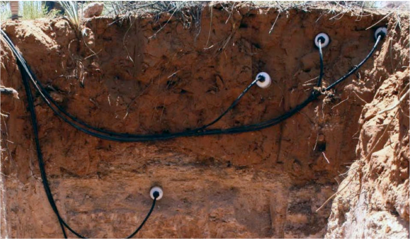
Figure 11 / Soil sensors installed in an inceptisol soil with a Bw horizon typical in a cambic epipedon. Picture compliments of the USDA NRCS SNOTEL Program.
