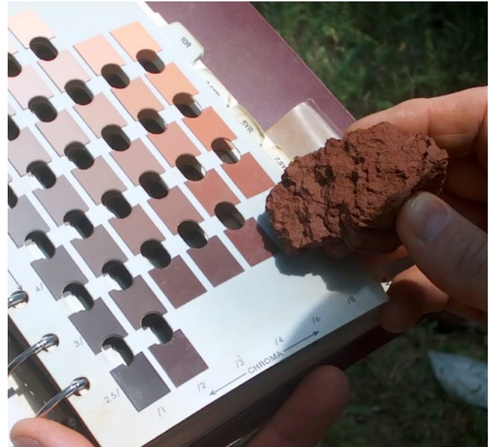
Figure 5 / Munsell Color book for identified soil colors and also a good field method for identifying soil horizons. Picture provided by the USDA NRCS.
